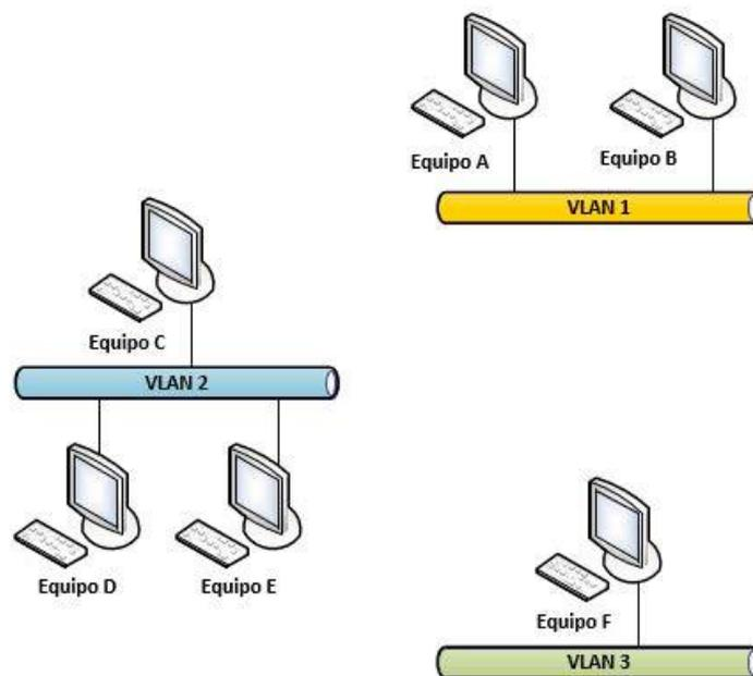
Figure 2: Network outline with computers connected to different VLANs
